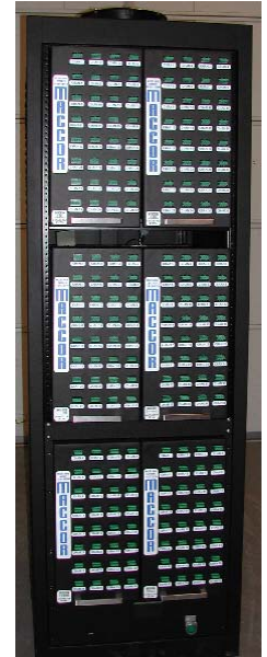
192 position model 3600 shown with Phoenix connector interface
